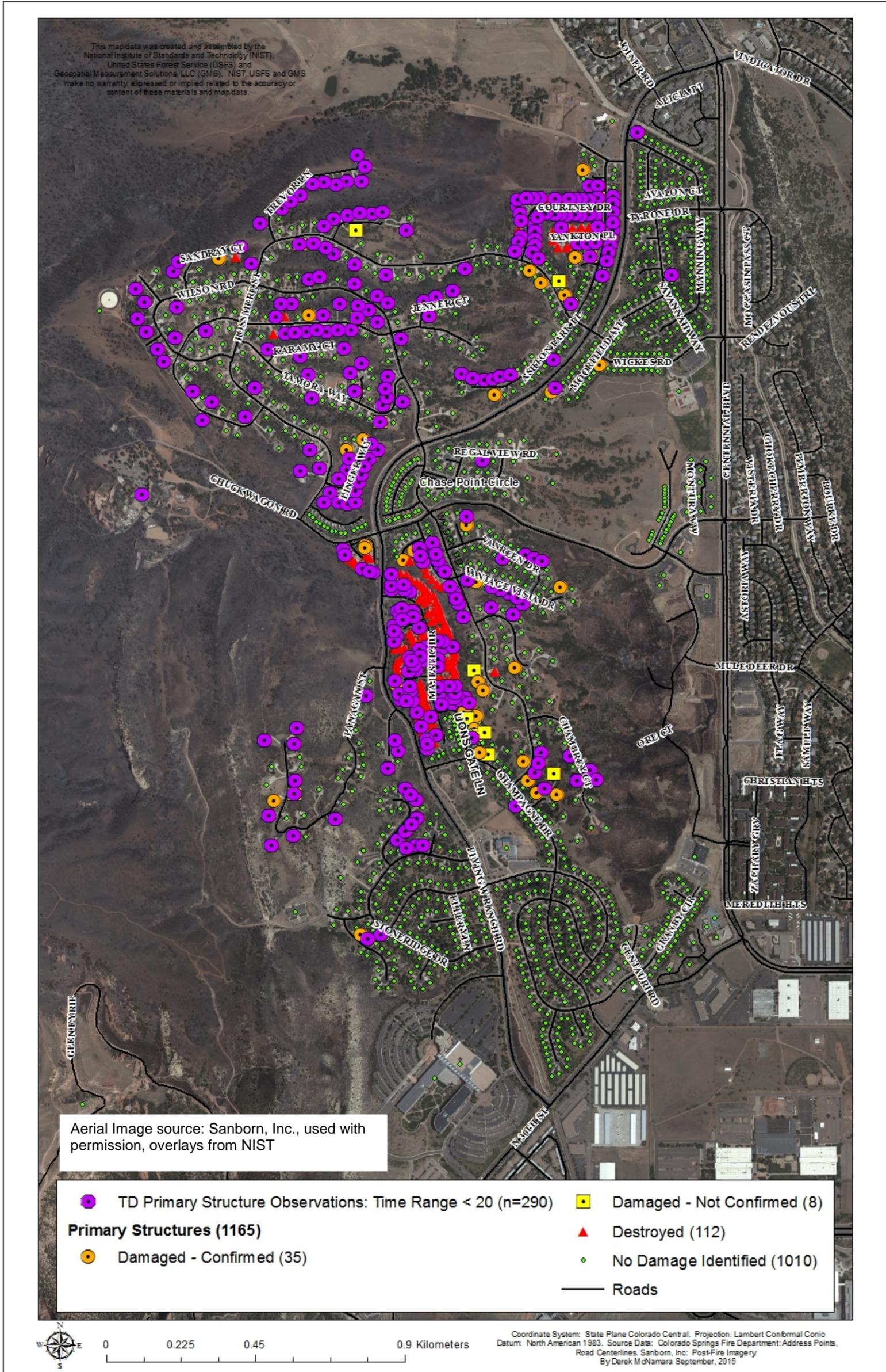
Map Figure 8 Primary structures with burn observations from TDs with time range estimates less than  $\pm 20$  min.
