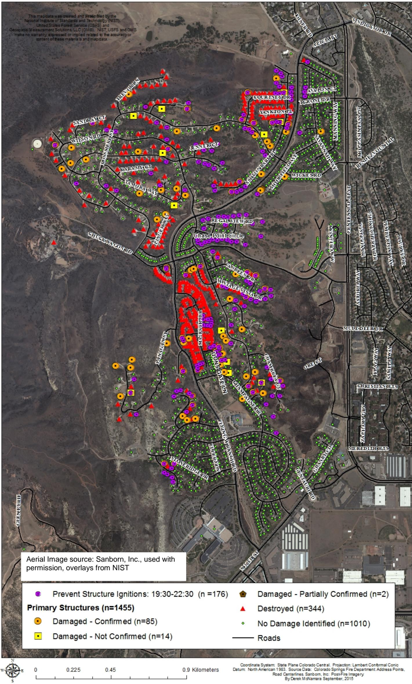
Map Figure 9 Primary structures identified as defended to “prevent structure ignition” between 19:30 and 22:30 overlaid on damage and destruction.
