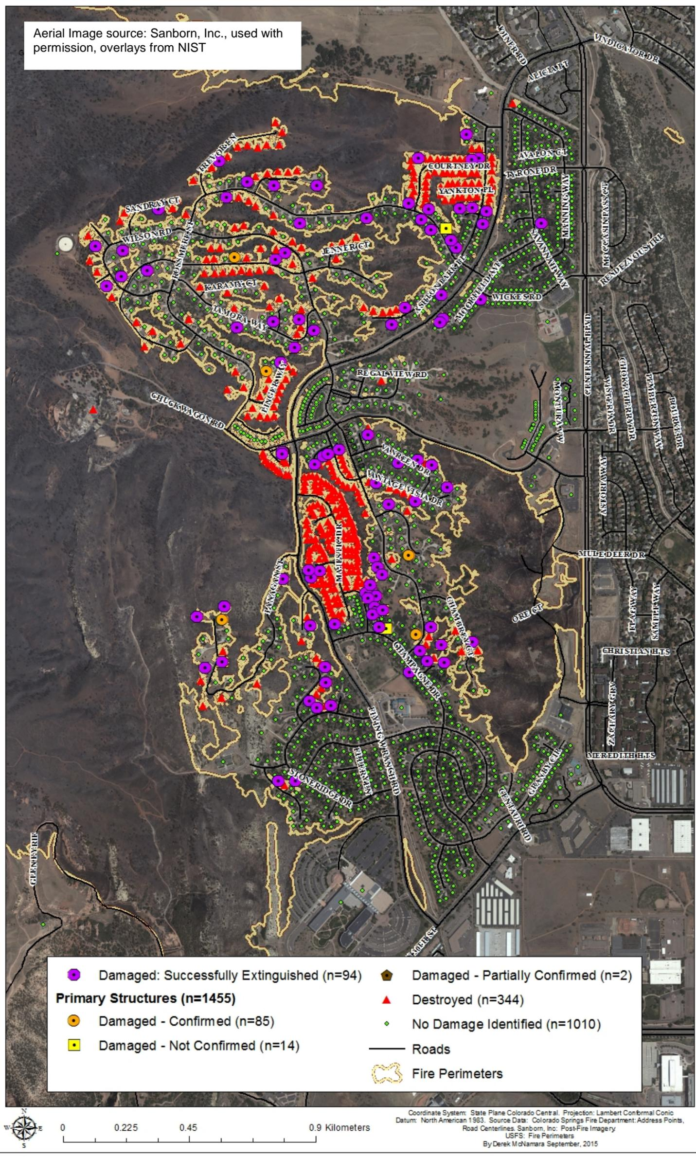
Map Figure 30 Structures with confirmed and possible damage, shown as purple hexagon with black dot, which were specifically identified by first responders as being extinguished (94/104 total or 93%).
