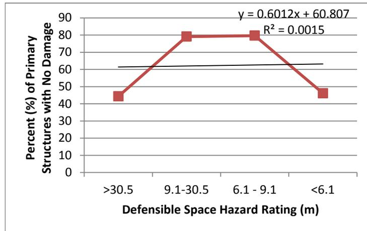
**Figure 56 Percent primary structures with no damage from the Waldo Canyon Fire by defensible space rating for all properties with a primary structure, a rating and a defensive action.**
