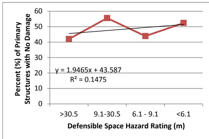
**Figure 55 Percent primary structures with no damage from the Waldo Canyon Fire by defensible space rating for all properties with a primary structure, a rating and no defensive actions as identified in this report.**
