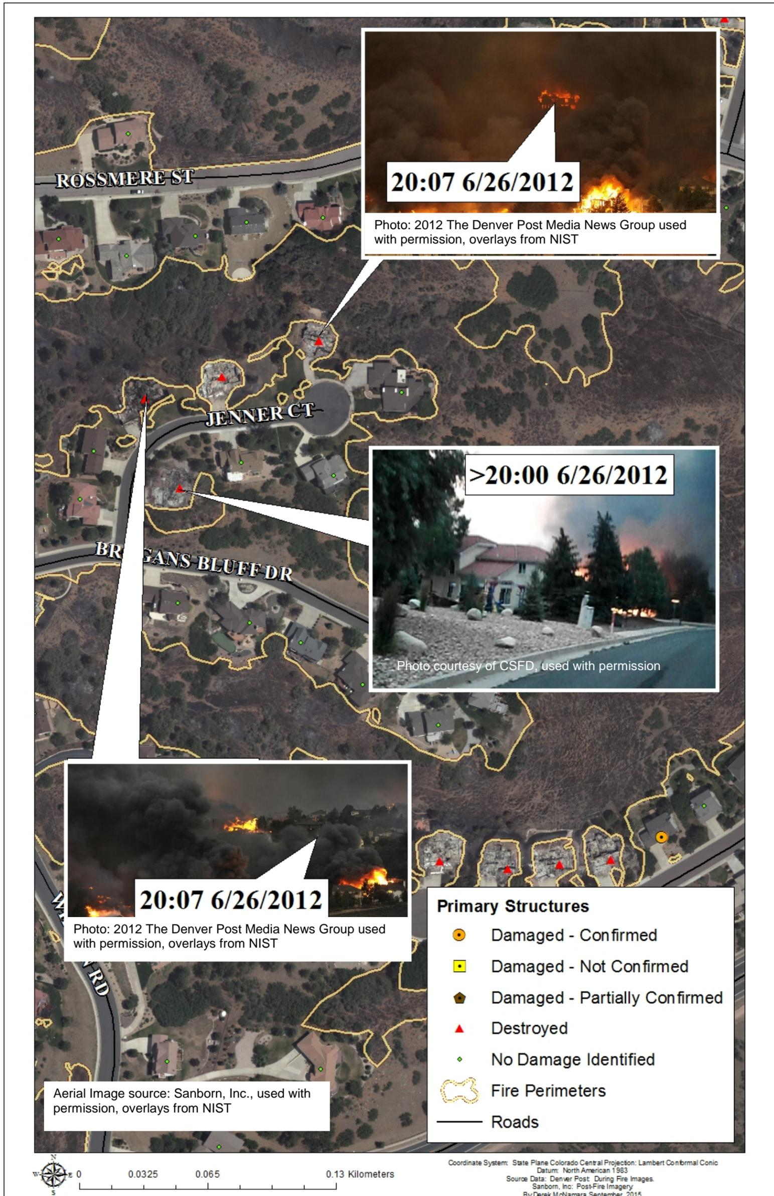
Map Figure 21 Structure ignitions on Jenner Court corresponding to changes in wind direction around 20:00.
