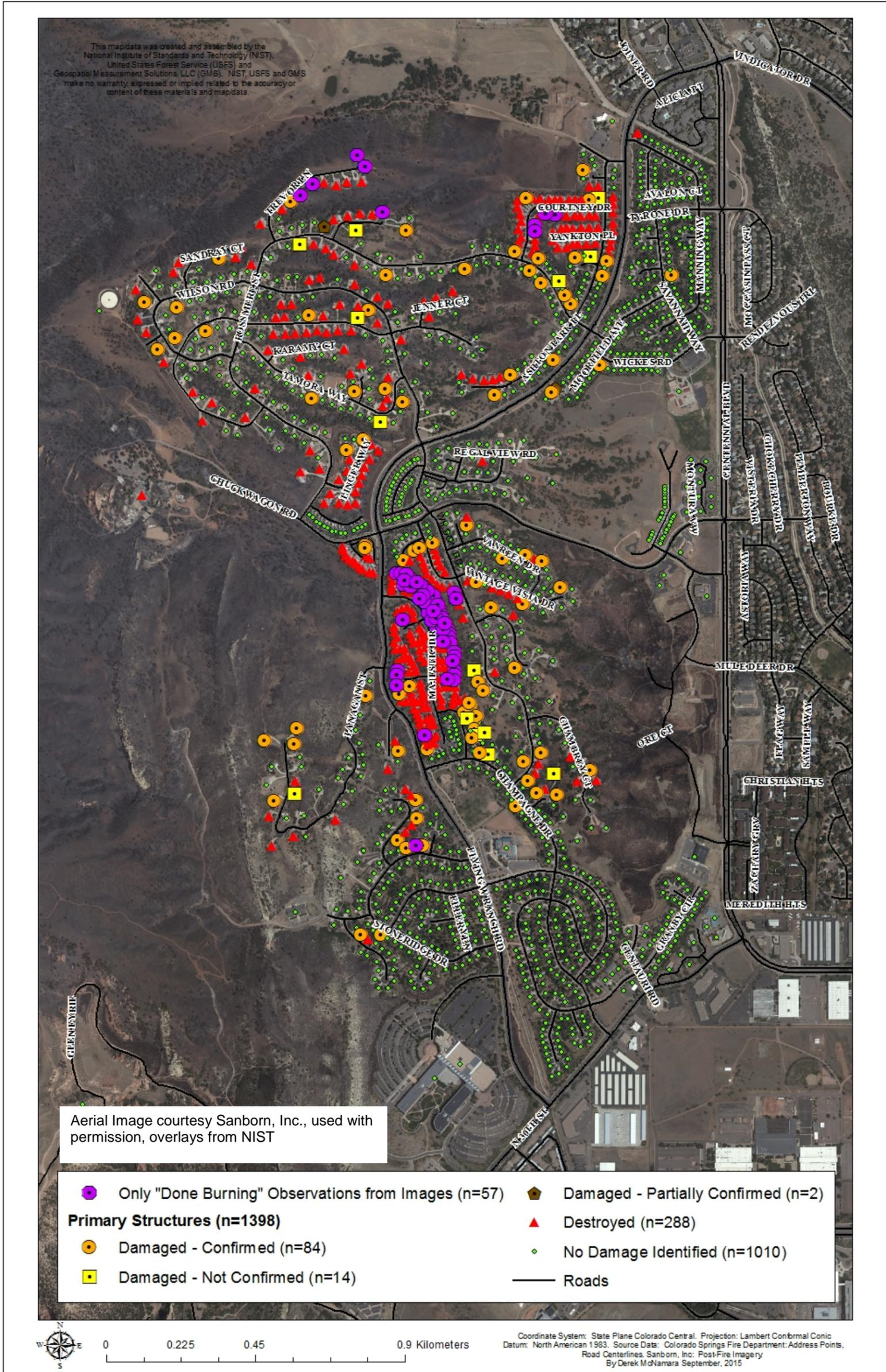
Map Figure 5 Primary structures with only "Done Burning" observations from images or videos overlaid on other primary structure damage categories.
