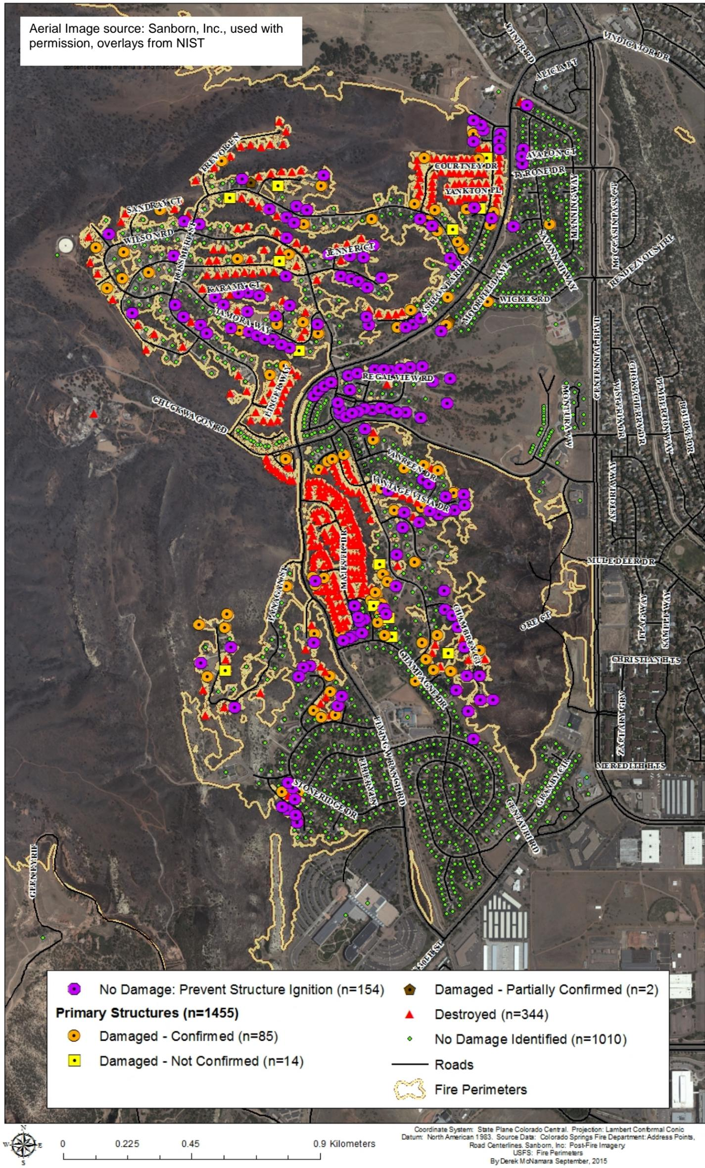
Map Figure 29 Structures with no damage, shown as purple hexagon with black dot, which were specifically identified by first responders as being defended to prevent structure ignition.
