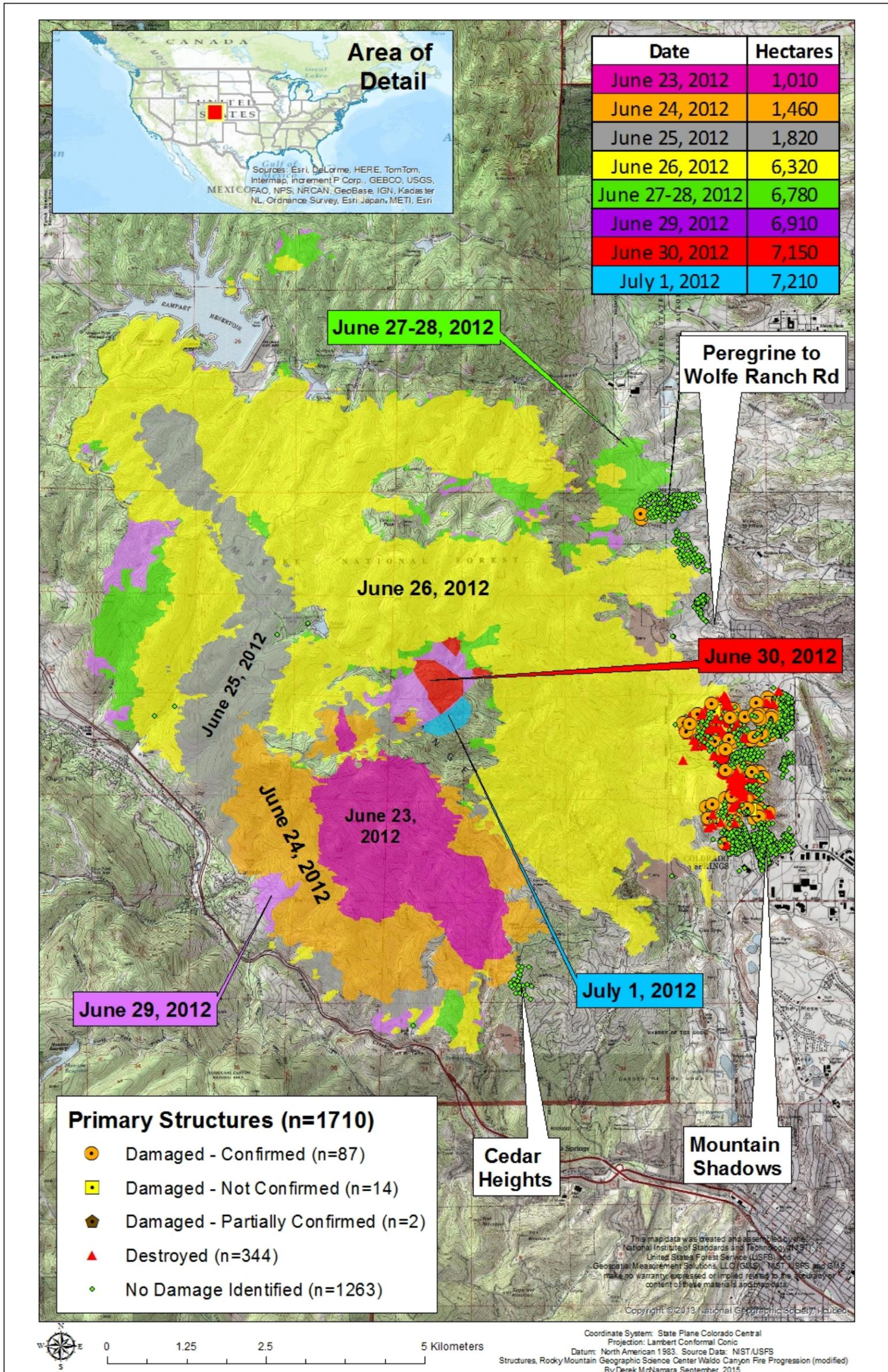
Map Figure 1 Fire progression of the 2012 Colorado Waldo Canyon Fire overlaid on structure response to the fire for primary structures in and around the fire.
